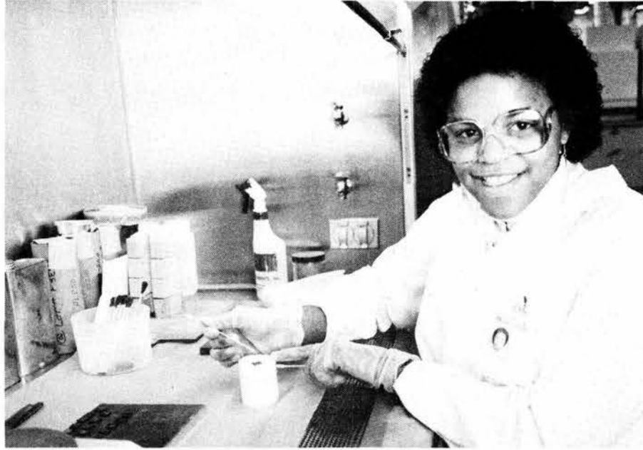
STICKING TO THE JOB — Working in the plastics lab on a project for Charlie Carter (7472-2), Tammie Jones (7472) bonds stainless steel pins to ferrite caps.
